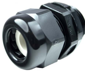
Large Compression Fitting for Patch Compartment Supports Cable O.D.: 0.59"-0.99" (P/N: CF-LG)
